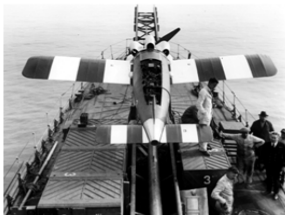
Figure 6 Larynx No3, the catapult from the HMS Stronghold destroyer on the 19th of October 1927 13
