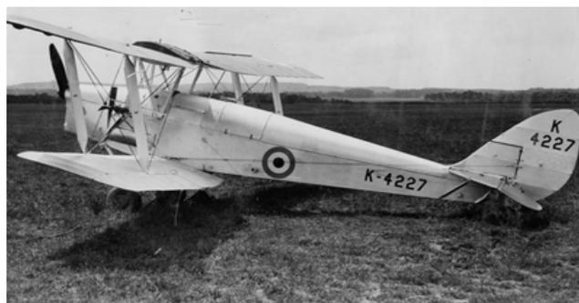
Figure 7 *The radio-controlled plane D.H.82B Queen Bee<sup>15</sup>*
