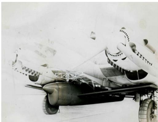
Figure 11 *Fi.157 drone attached to an He 111*<sup>22</sup>
