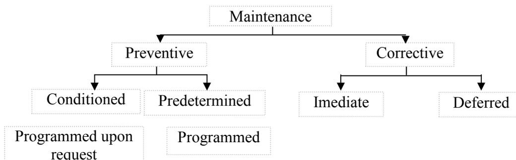
**Fig. 1** Maintenance types according to EN 13306: 2001
