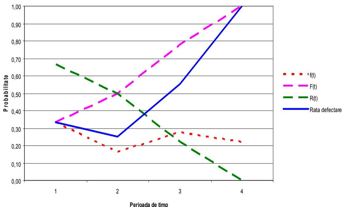
**Fig. 2** Failure model basic functions
