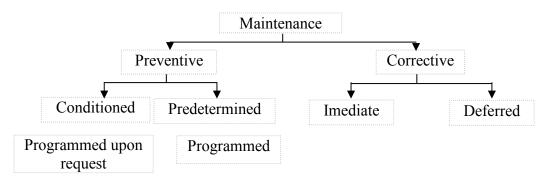
Fig. 1 Maintenance types according to EN 13306: 2001
