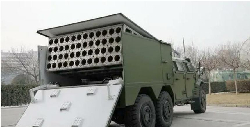
**Figure nr. 7:** The “Hummer” – type vehicle with 48 UAV launching tubes
